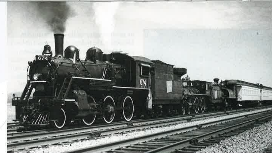
CN's 19th-century heritage is represented by three locomotives leading the railroad's museum train in 1956. On the point is a 2-6-0 built in 1899 at CN's Point St. Charles Shops in Montreal, followed by a 4-4-0 built in Portland, Maine, for the Grand Trunk in 1872, and an 0-6-0 saddle-tank switcher built at Point St. Charles in 1894. Canadian National
